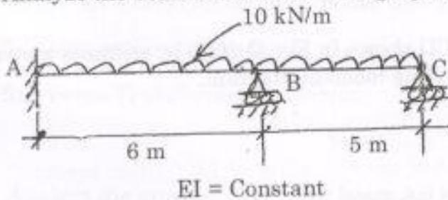
15. a) Analyze the beam ABC shown in Fig. Q 15 (a) by stiffness method.
