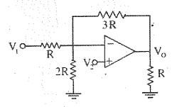
(ii) For given circuit the operational amplifiers are ideal find out the output voltage Vo. (5)
