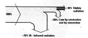
The above is the Sankey Diagram of which lighting system? What is the efficiency of this system? Comment on this value and propose a modern replacement of this system. Name the proposed system and state its advantages and disadvantages with compared to the above, in terms of efficiency, efficacy, cost, working or burning hours (life), CRI, etc. What is the trend and future of lighting systems at home, streets and industries?
