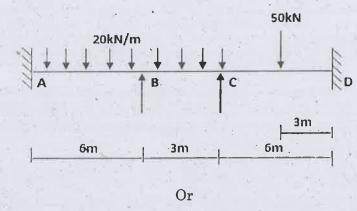
(b) Analyse the continuous beam loaded as shown in fig. by moment distribution method and find final moments.
