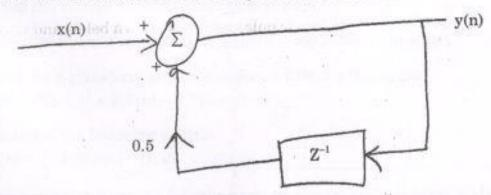
Find the frequency response  $H(e^{i\omega})$  and the impulse response h(n) of the system. Sketch the magnitude response  $|H(e^{i\omega})|$  for the system.
