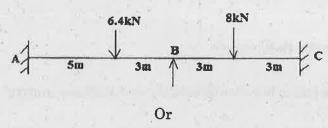
(b) Analyse the given frame by stiffness matrix method.
