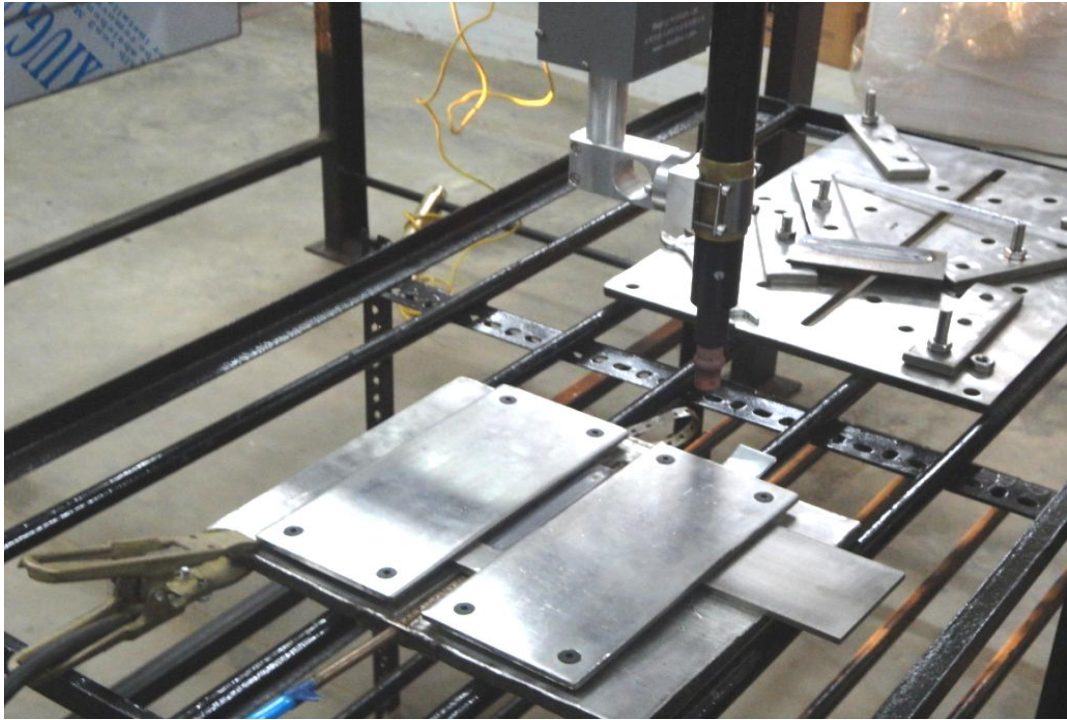
Fig 6.1 Robotic TIG Welding set up
