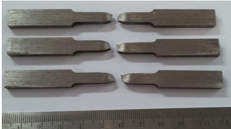
Fig 7.1.2: Welded sample after Tensile Test
