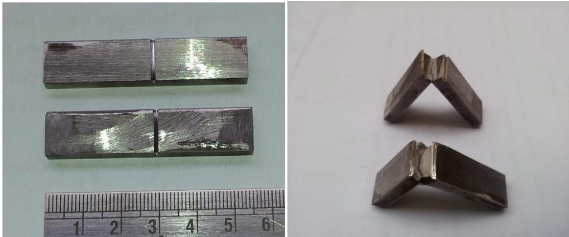
Fig 7.2: Welded sample after Impact test
