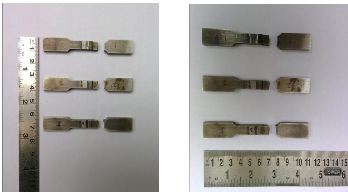
Fig 7.3: Welded sample after Fatigue Test
