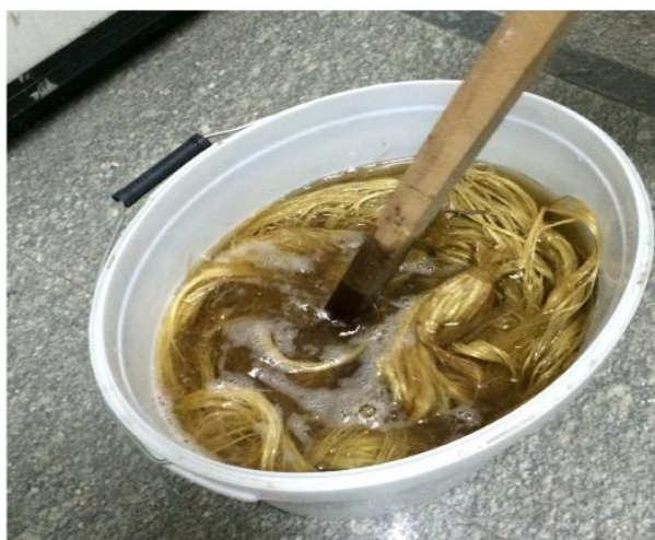
Fig.3.4. Alkali (NaOH) treatment of Banana Stem Fibres
