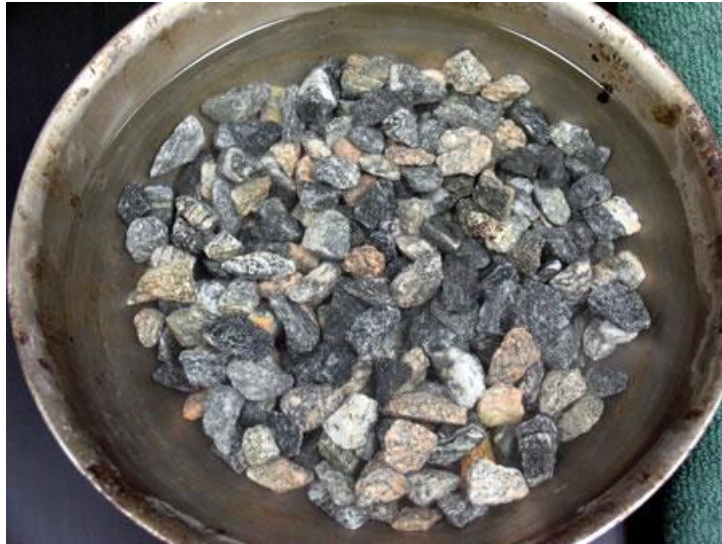
Fig.4.1. Water Absorption Test on Aggregate
