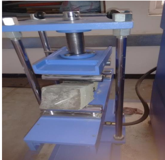
Fig 4.7 Testing of beams in flexural testing machine
