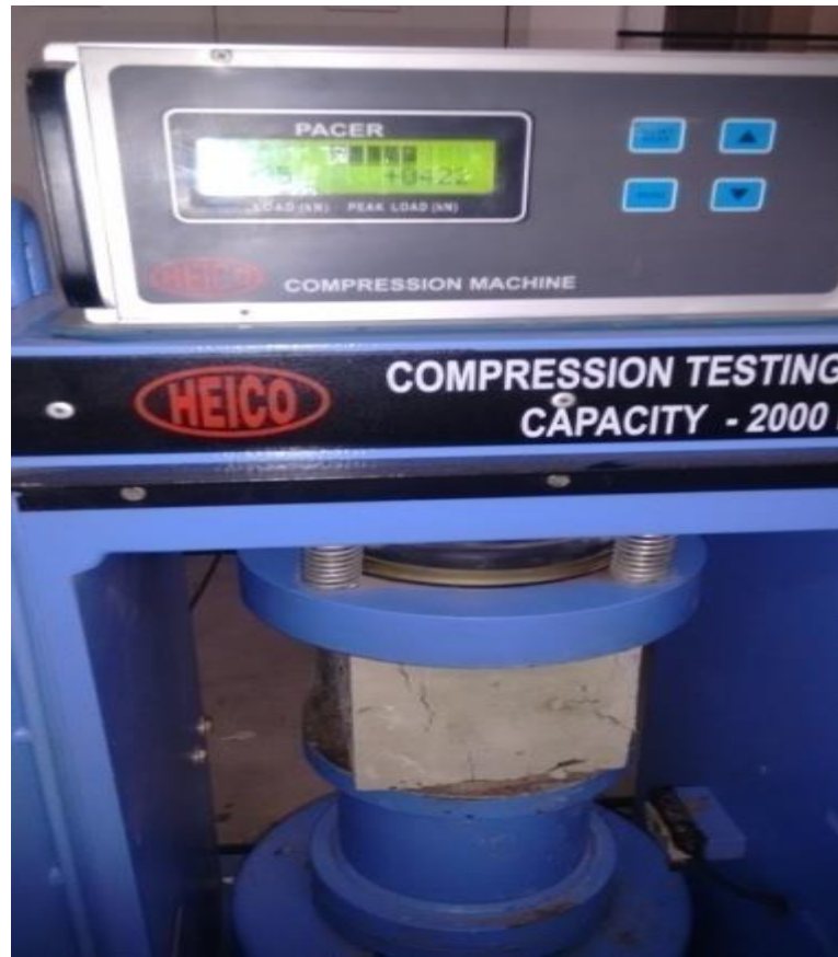
Fig 4.5 Testing of cubes in CTM
