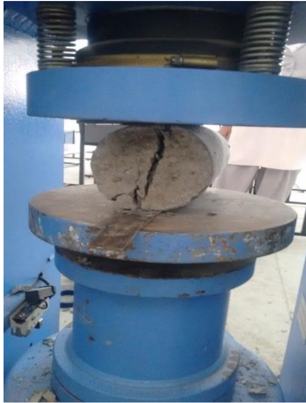
Fig 4.6 Testing of cylinder in compression testing machine.
