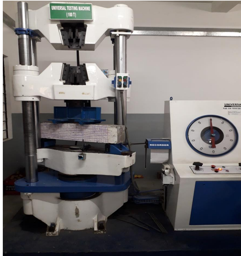
Fig 12: Flexural and Shear Strength test(UTM)
