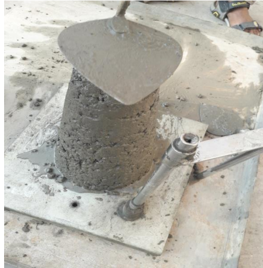
Fig 11: Slump Cone test
