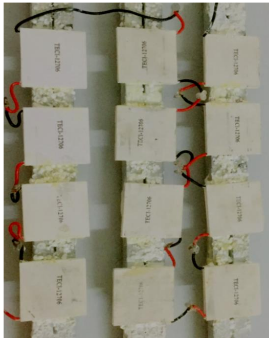
Fig. 2.5 Series configuration of the system
