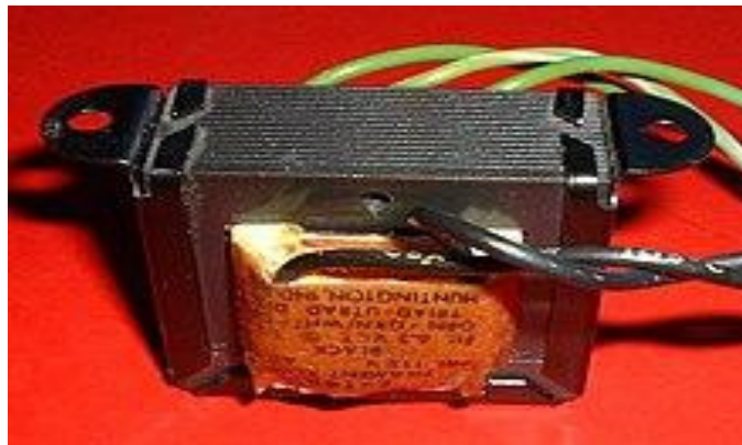
Fig 3.2 Single phase transformer
