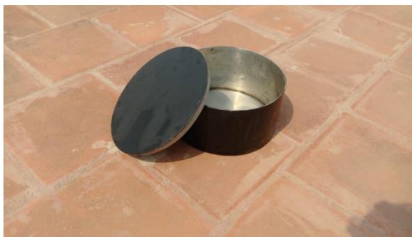
Figure 3.3 Mild steel Pan
