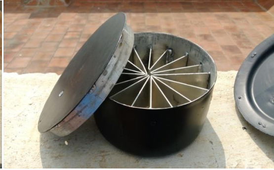
Figure 3.6 Aluminium pan with Internal fins
