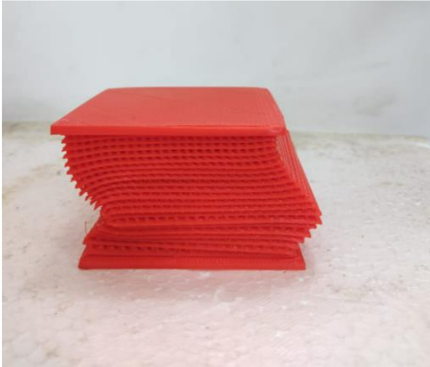
Fig 25: FGM Foam After Compression Test
